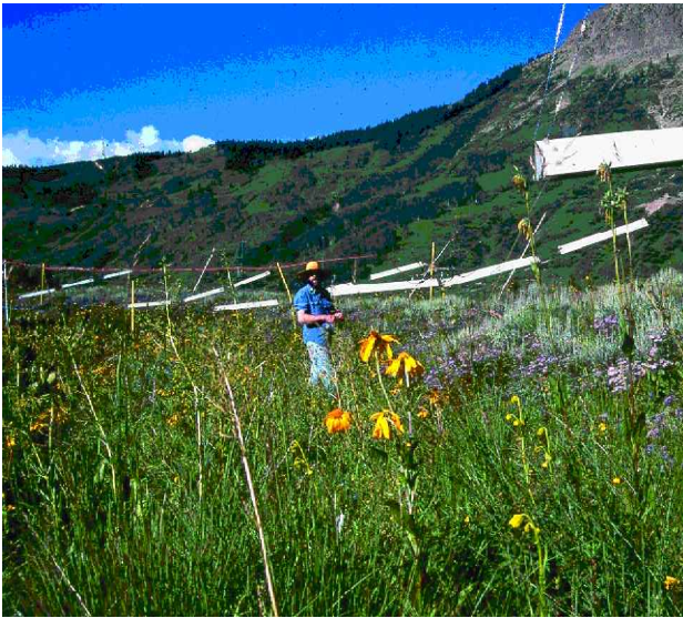
Figure 6. Infrared heaters in place above subalpine meadow vegetation, Colorado. Photo: Taylor Ricketts.
